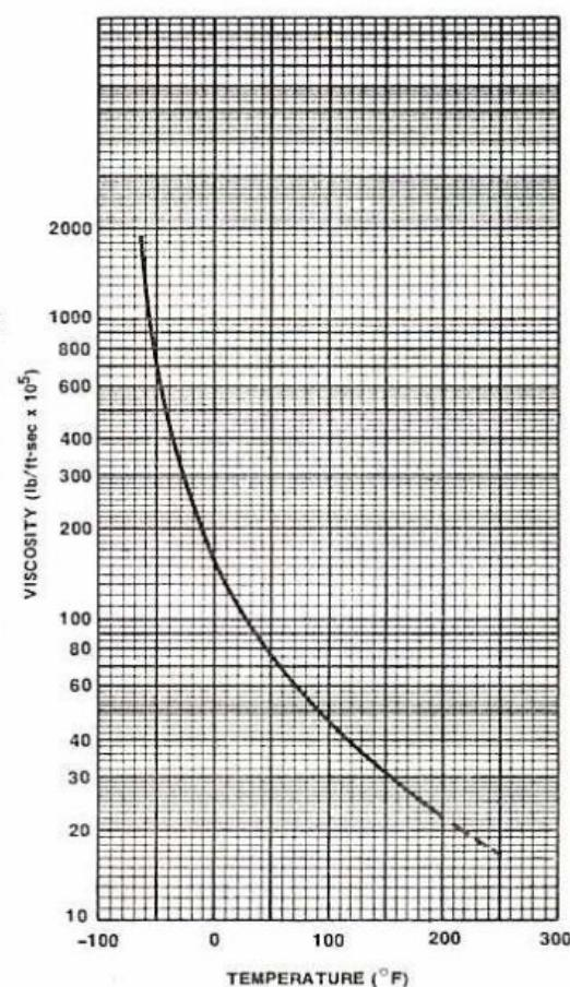
PHYSICAL PROPERTIES OF MHF-3: 86% MMH - 14%  $N_2H_4$ , b.w.
