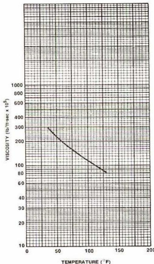
PHYSICAL PROPERTIES OF MAXIMUM DENSITY INHIBITED FUMING NITRIC ACID:
